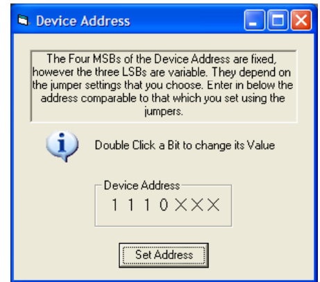
Figure 3. I 2 C Address Selection
